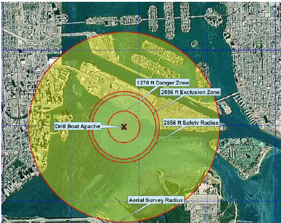
**Figure 3 – Sample zone layout using the mean weight of explosives of 119lbs (53.98 kg).**
